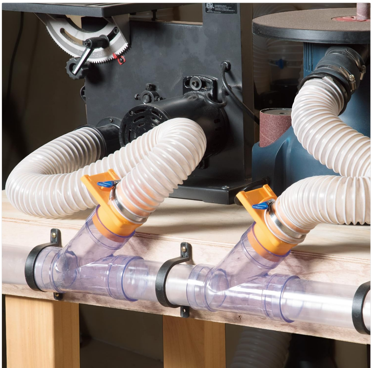
Figure 4: Example of a dust collection system layout.
