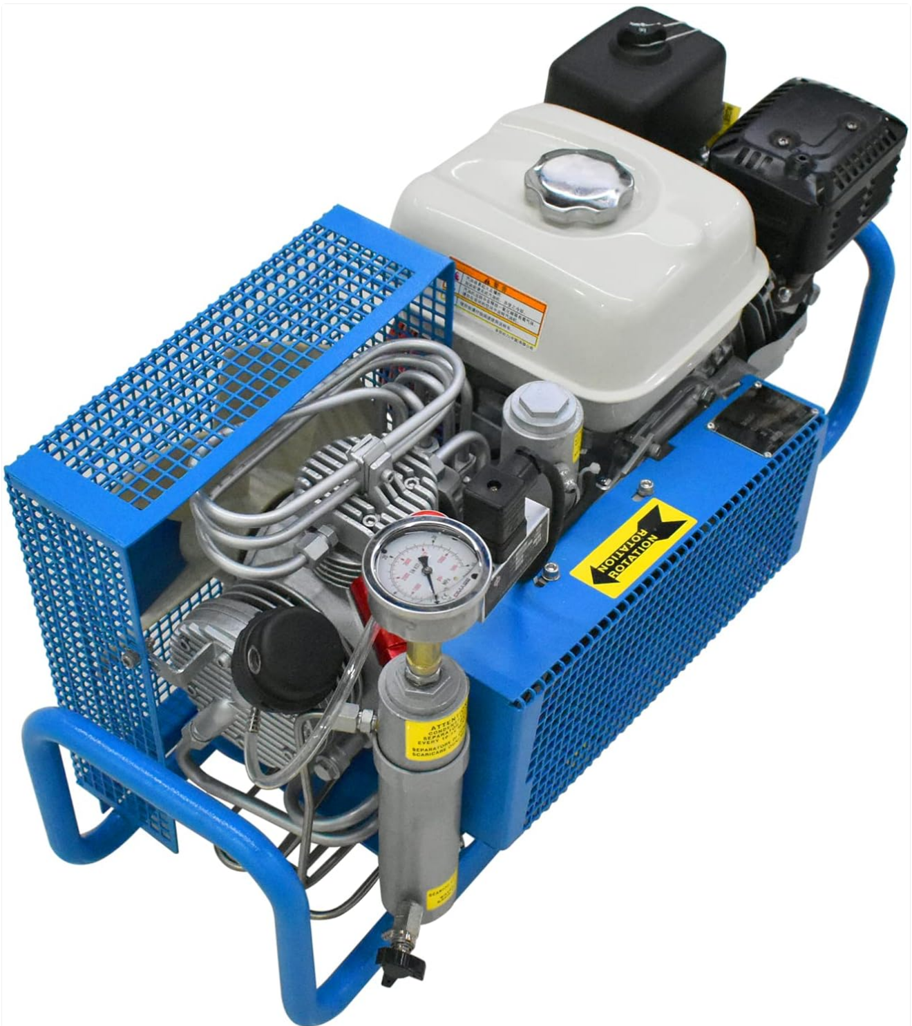
Figure 6.1: Top angled view of the compressor, showing the engine, compressor unit, and pressure gauge. This perspective helps in locating controls and monitoring during operation.
