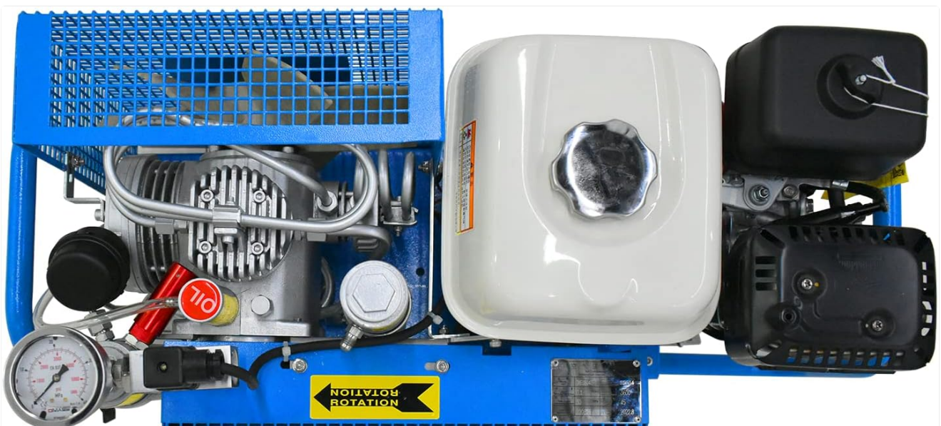
Figure 3.3: Top view of the compressor, providing a clear perspective of the engine, compressor block, and various connections from
