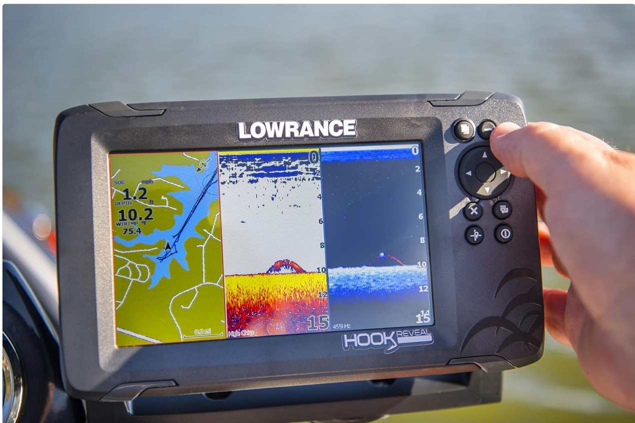
Figure 3.4: Lowrance HOOK Reveal display showing a split-screen view, combining C-MAP navigation with real-time sonar data.
