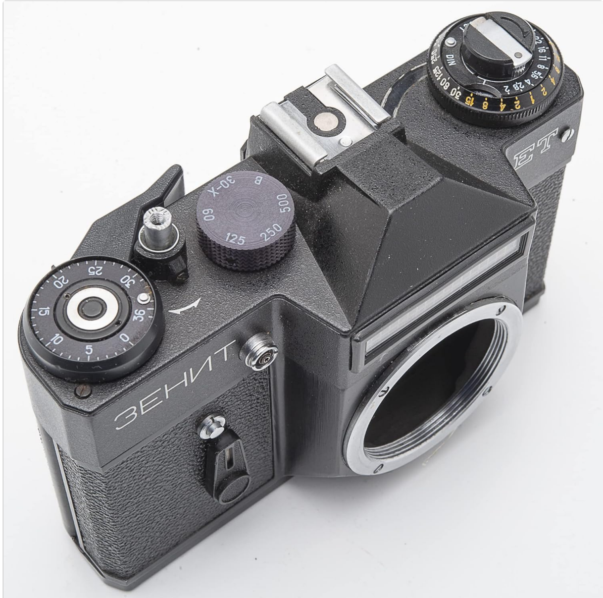
Image: Top view of the Zenit ET camera body, highlighting the controls on the top plate including the film advance lever and shutter speed dial.
