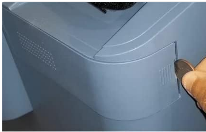
The Intake Filter Cover is located on the back of the EverFlo - The Intake Filter is behind the panel shown in the image above.
