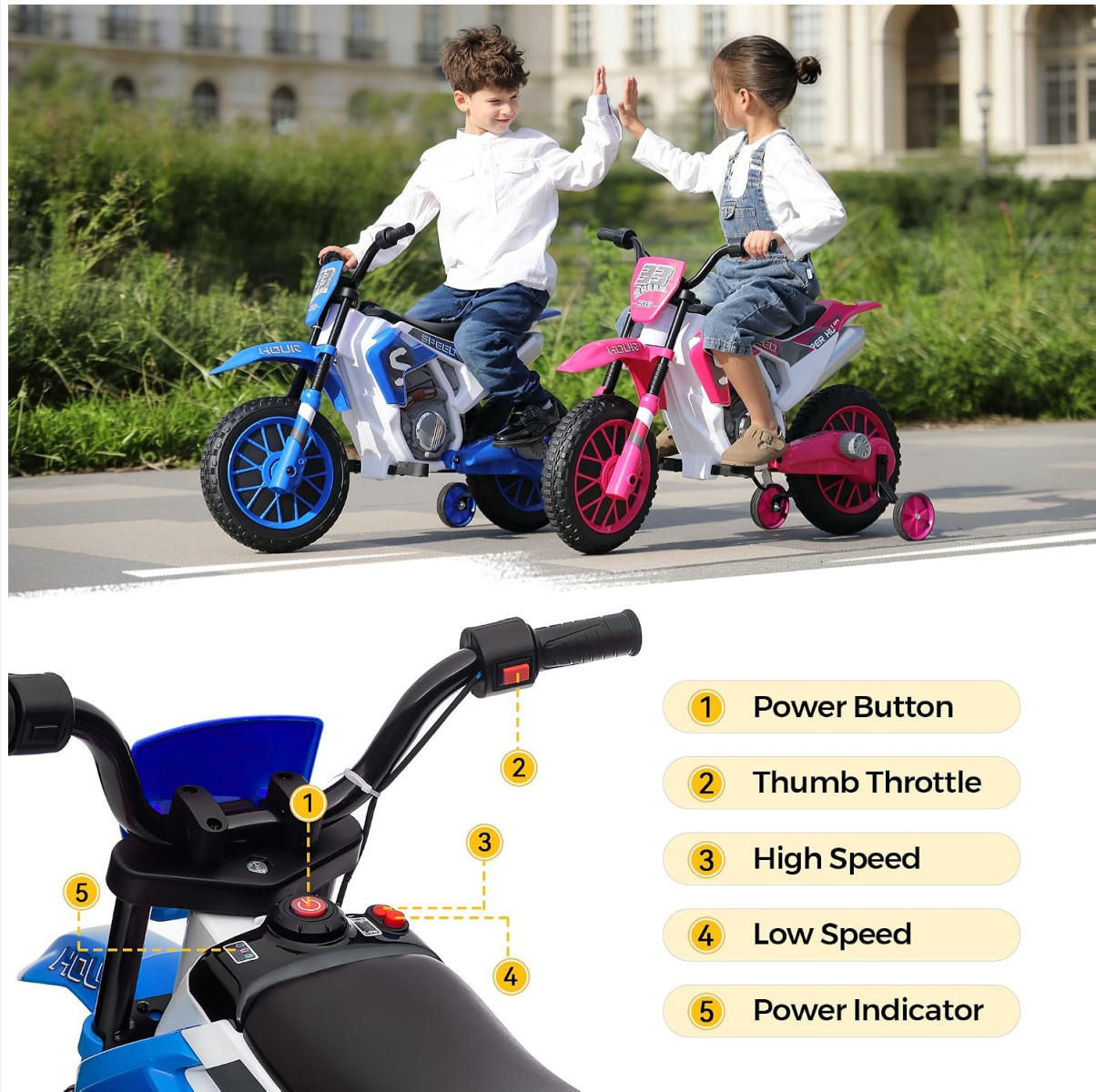
Figure 3: Control panel layout with key functions labeled.
