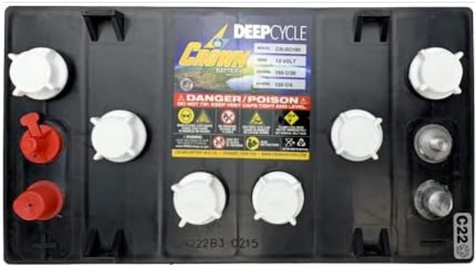
Image: Top view of a Crown CR-GC150 battery, illustrating the six removable fill caps and the SAE automotive post and threaded stud terminals for proper connection and maintenance.
