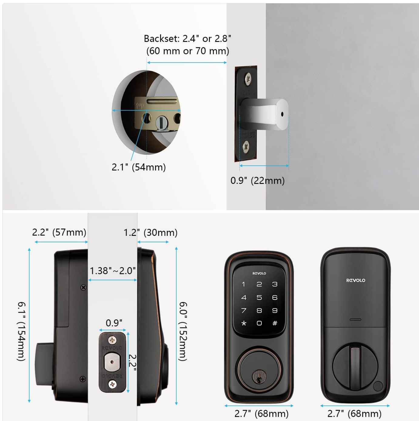
Image: A detailed diagram illustrating the dimensions of the Revolo Keyless Entry Door Lock components, including the exterior keypad, interior assembly, latch, and strike plate, along with measurements for door preparation.
