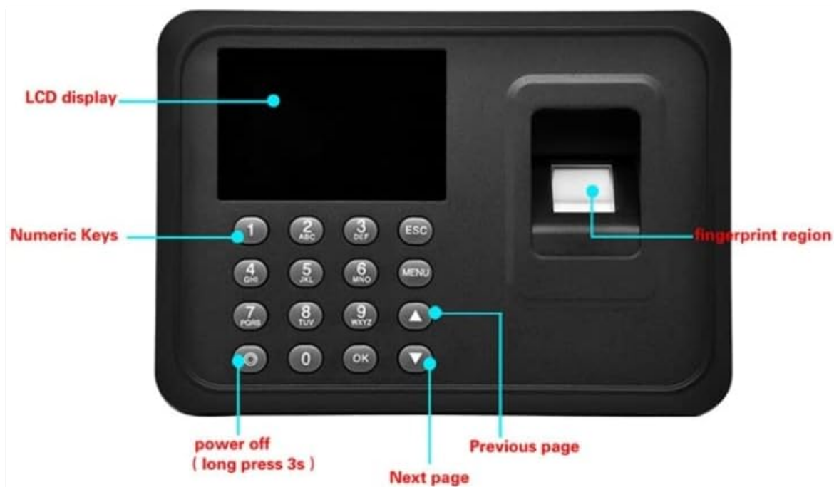
Image 2.2.1: Front view of the A6 Time Attendance Machine with key components labeled. This includes the LCD display, numeric keys for input, the fingerprint region for biometric scanning, and navigation buttons for menu control. The 'power off' button requires a 3-second long press to activate.
