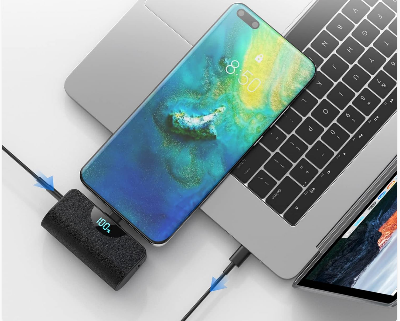
Figure 4.2: Pass-through charging setup.
