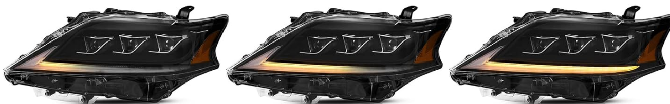
Image: Demonstration of the sequential turn signal indicator, showing the progressive illumination of the amber light bar.
