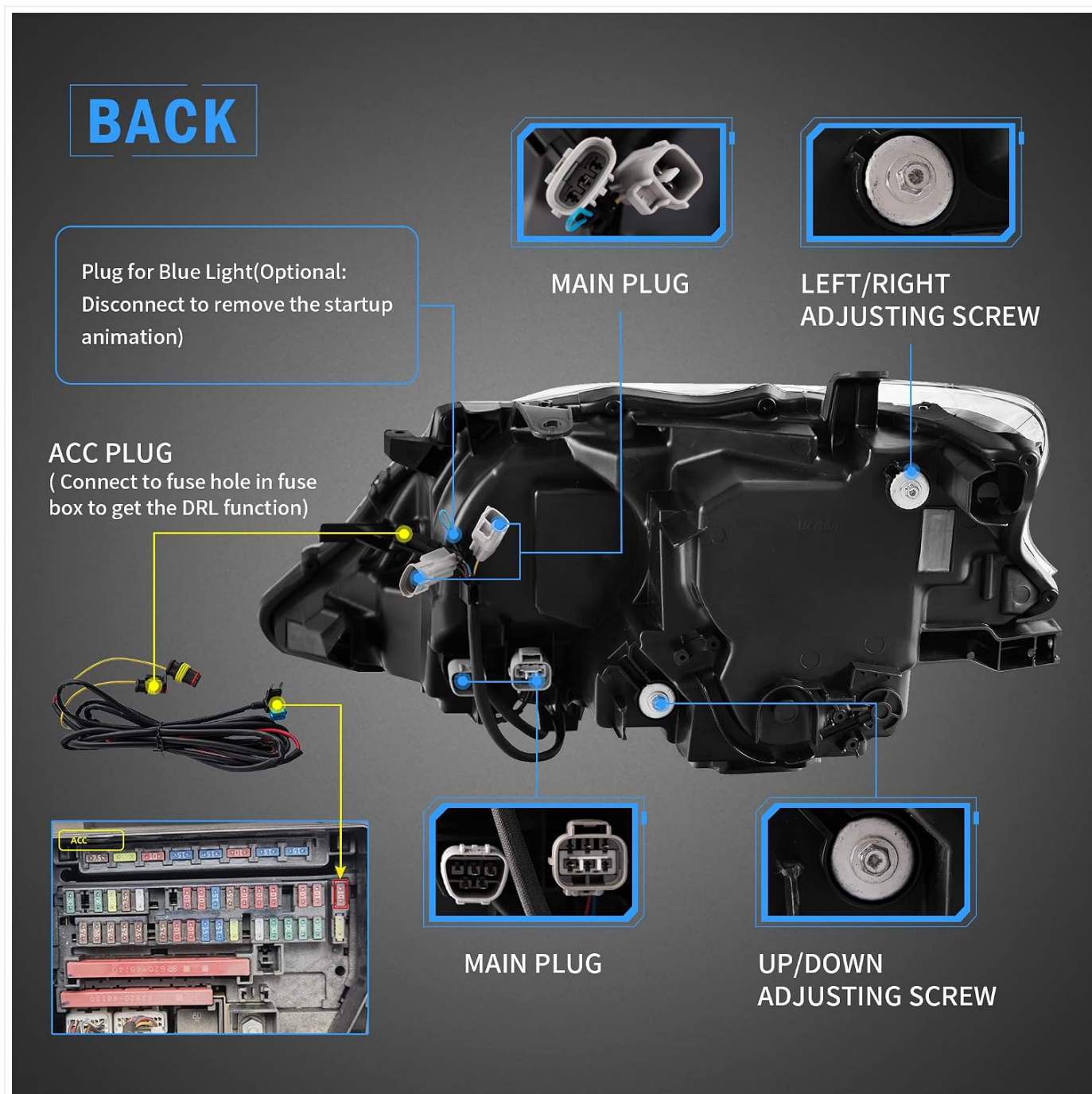
Image: Rear view of the VLAND headlight assembly, illustrating the main plug, ACC plug for DRL, optional blue light disconnect, and adjustment screws for light alignment.
