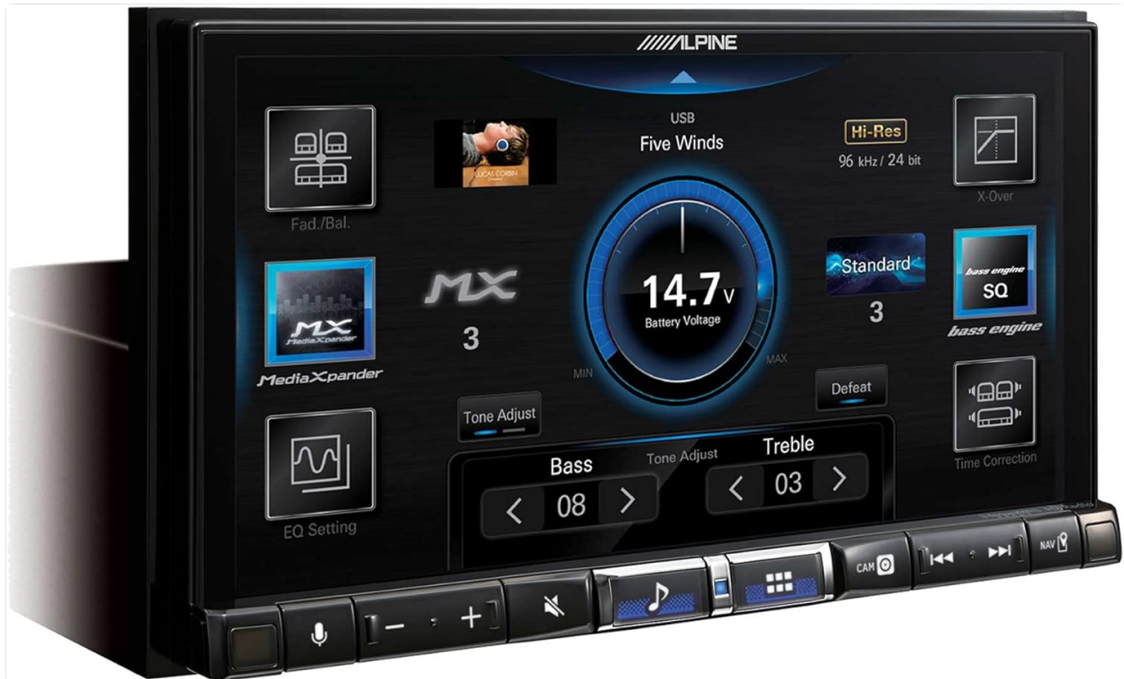
Figure 4: The audio settings screen of the Alpine iLX-507, showing options for MediaXpander, battery voltage display, sound presets, bass/treble adjustments, and time correction settings.
