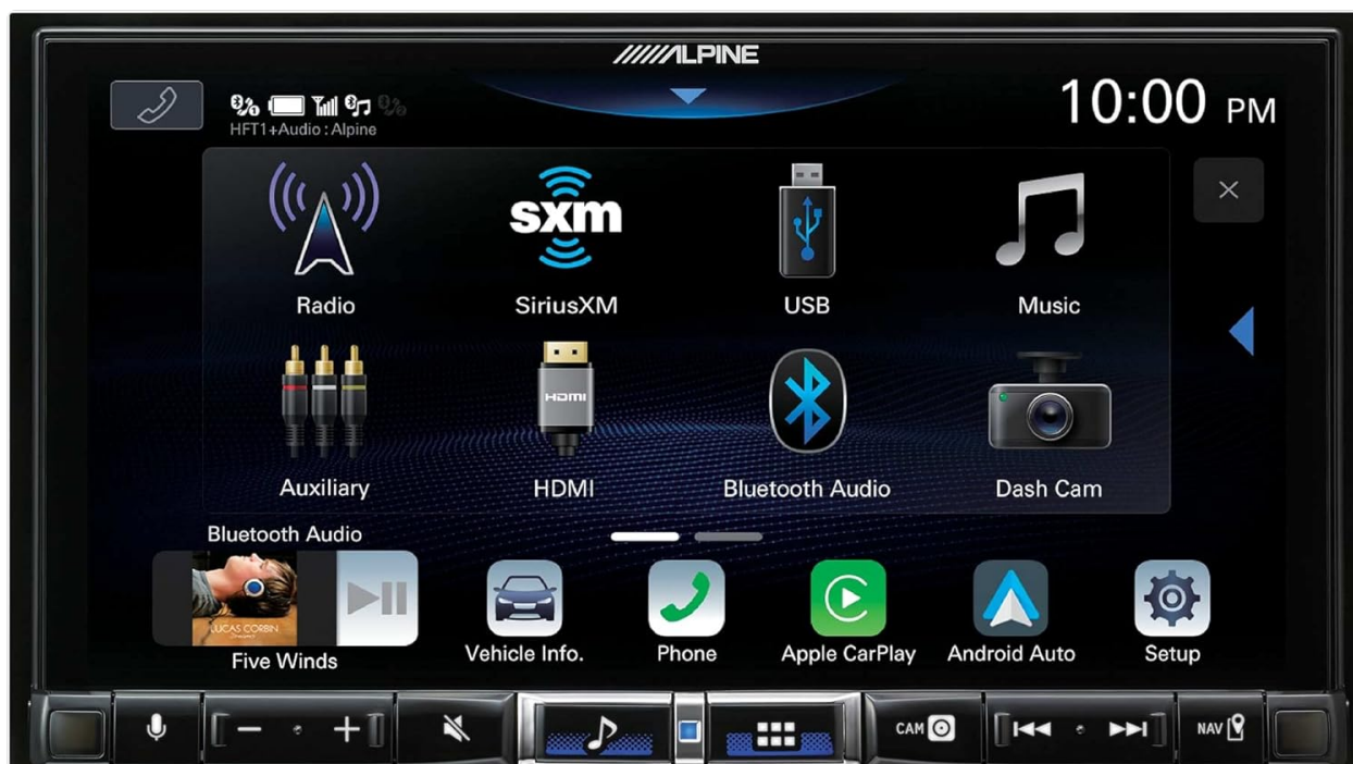
Figure 2: The main menu screen of the iLX-507, showing icons for Radio, SiriusXM, USB, Music, Auxiliary, HDMI, Bluetooth Audio, Dash Cam, Vehicle Info, Phone, Apple CarPlay, and Android Auto.
