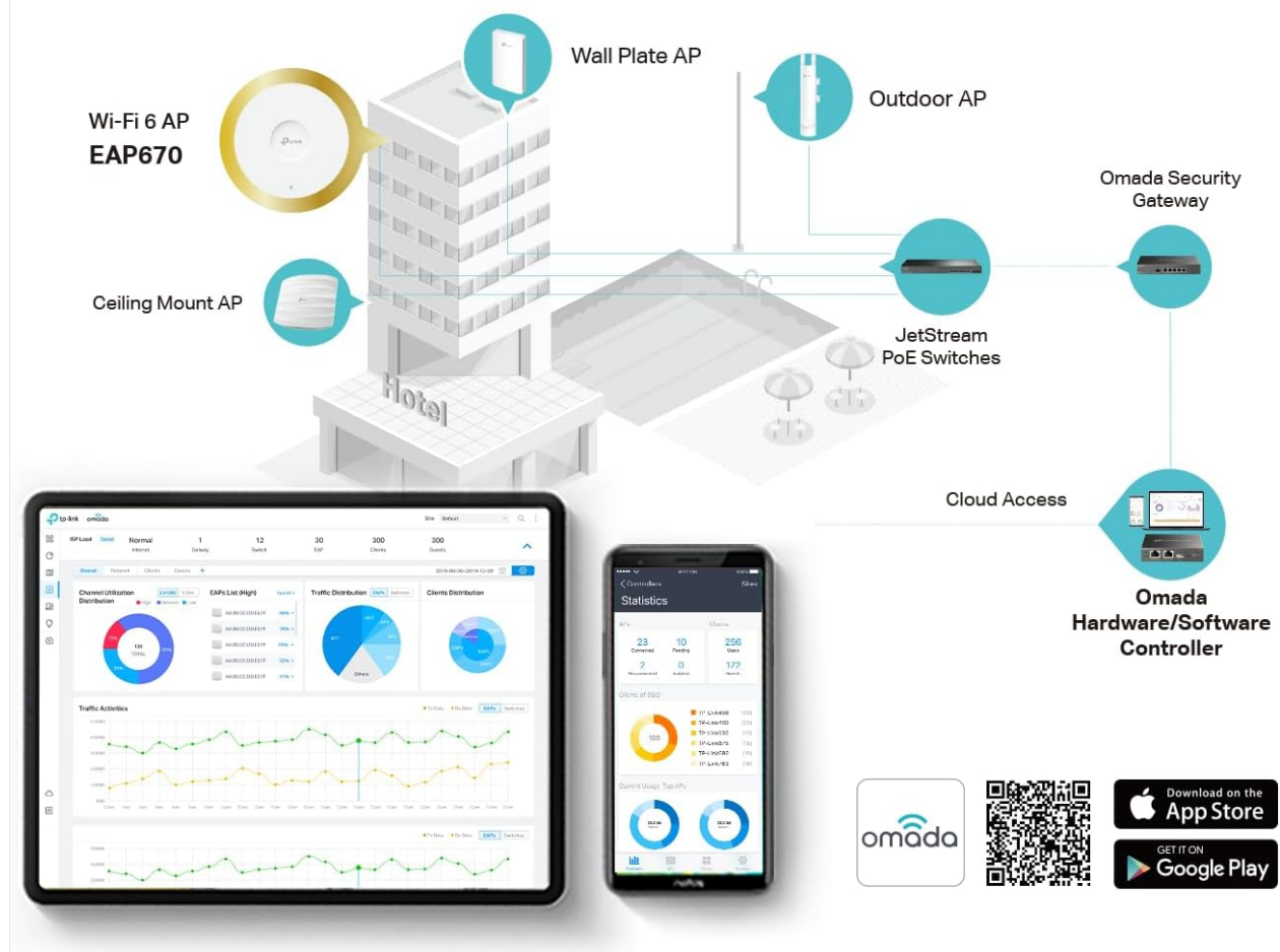
Image 5: Overview of the Omada cloud solution for business networking, demonstrating centralized management via tablet and smartphone apps, integrating various Omada devices.
