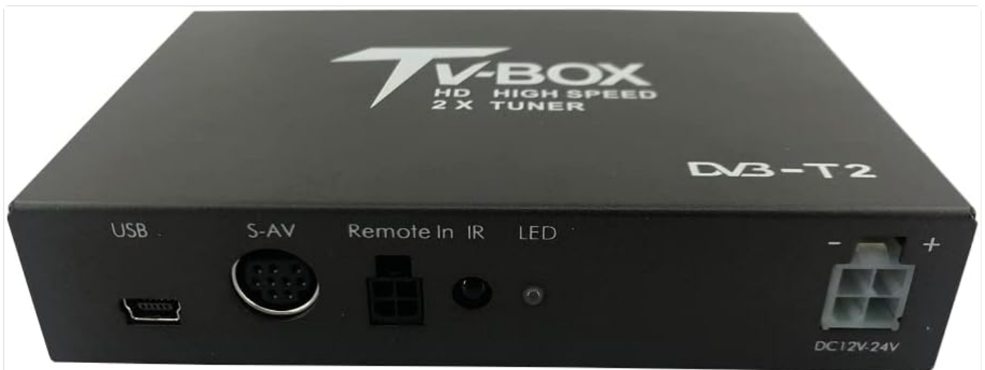
Image: Front panel of the receiver with the DC 12V-24V power input connector.
