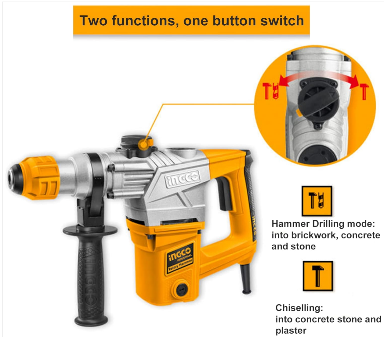
Figure 5.1: The function selector switch for Hammer Drilling and Chiseling modes.
