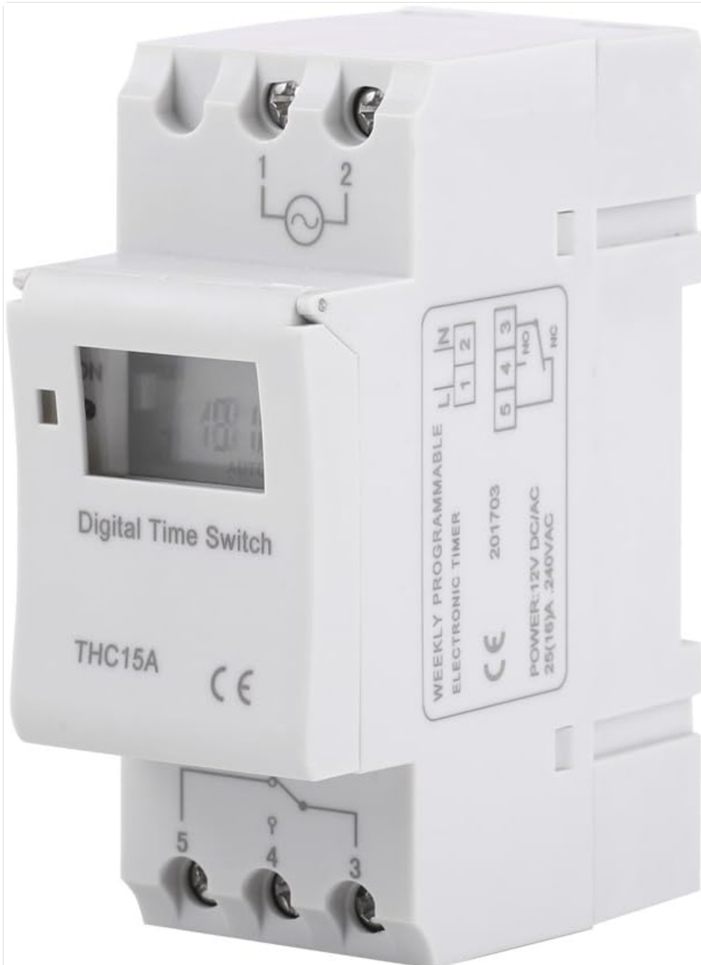
Figure 7.1: Wiring Diagram. Terminals 1 and 2 are for power input (L and N). Terminals 3, 4, and 5 are for output control (NO, Common, NC).
