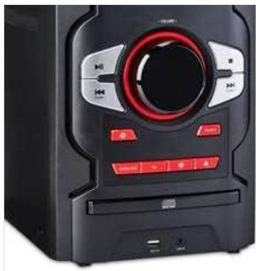
Image: A close-up view of the main unit's front panel, highlighting the central volume knob, playback controls, equalizer buttons, LED light mode buttons, CD tray, and USB charging port.
