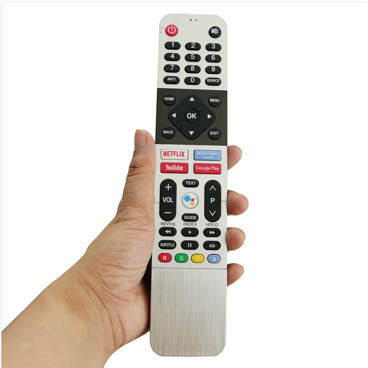
Image: Front view of the remote control, illustrating its design and highlighting features such as four dedicated shortcut keys for streaming services (Netflix, Prime Video, YouTube, Google Play), soft plastic buttons, durable ABS material, and the "no need to set up" functionality.
