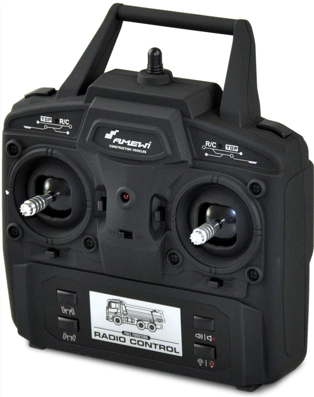
Image 4.2: The 2.4 GHz remote control for the Amewi 22533 dump truck.
