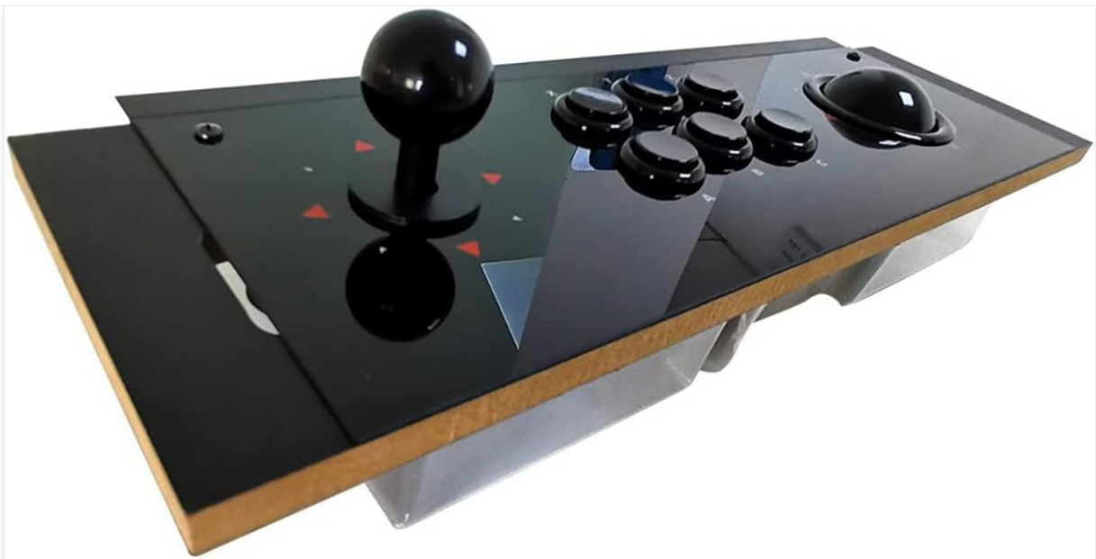
Figure 4.1: The AtGames Arcade Control Panel, featuring an 8-way joystick, multiple action buttons, and a trackball controller.
