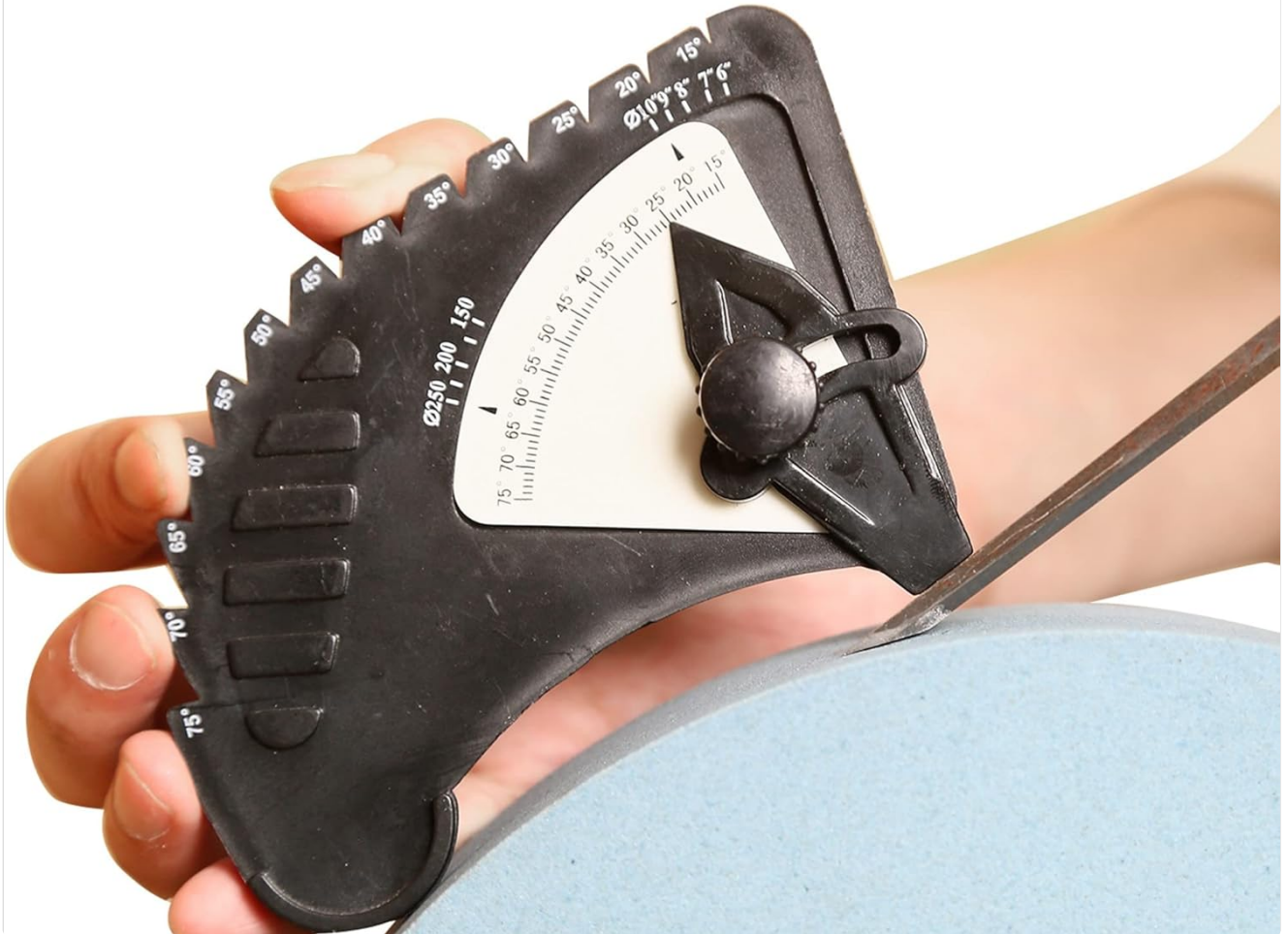
Image: A hand demonstrating the use of the angle guide for precise sharpening on the wet stone.
