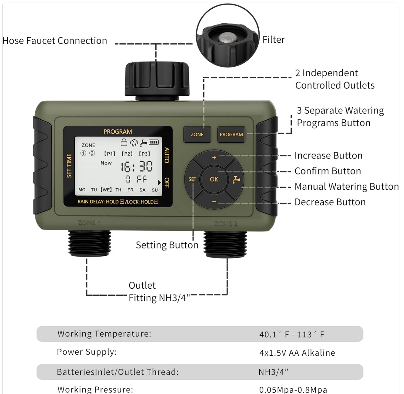
Figure 1: Diivoo 2-Zone Sprinkler Timer Components. This diagram illustrates the main parts of the timer, including the hose faucet connection, filter, independent controlled outlets (Zone 1 and Zone 2), setting button, increase/decrease buttons, OK button, manual watering button, and program buttons. It also lists specifications such as working temperature, power supply, batteries/inlet/outlet thread, and working pressure.
