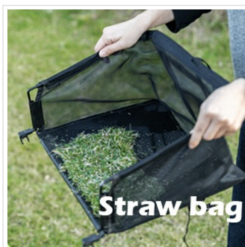
Figure 4.4: The grass catcher, ready for use or emptying.
