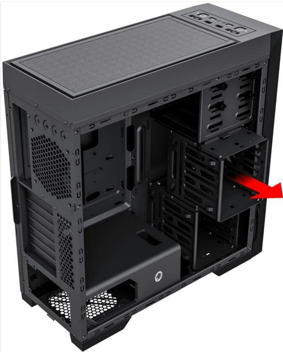
Figure 2: Interior view showing the removable drive cages for 3.5" HDDs.
