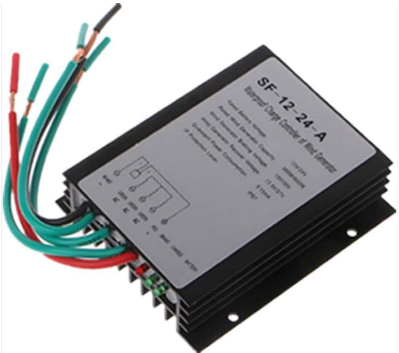
Figure 5.3: The Giosolar SF-12-24-A Wind Charge Controller, showing its input and output terminals for connecting to the wind turbine and battery bank.
