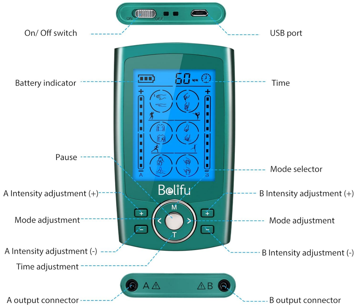
Figure 3: Overview of the device's buttons, ports, and display indicators.
