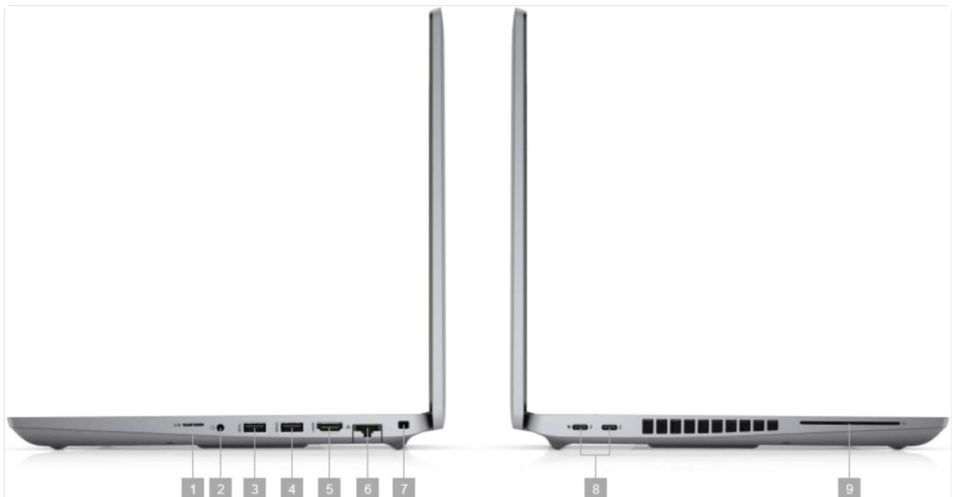
Image: Right side view of the Dell Latitude 5521 Laptop. This image highlights the ports located on the right side of the laptop, such as USB-C ports and the SD card reader.
