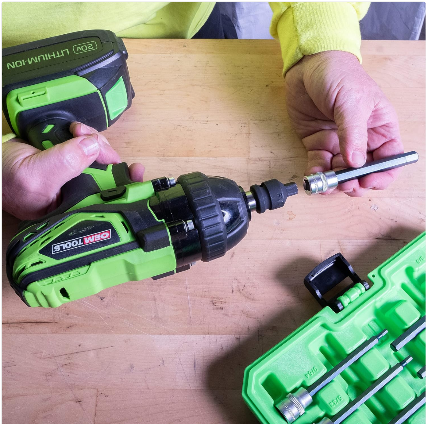
Figure 6: A user demonstrating the insertion of a hex bit socket into an impact driver, showcasing the compatibility of the sockets with power tools for efficient operation.
