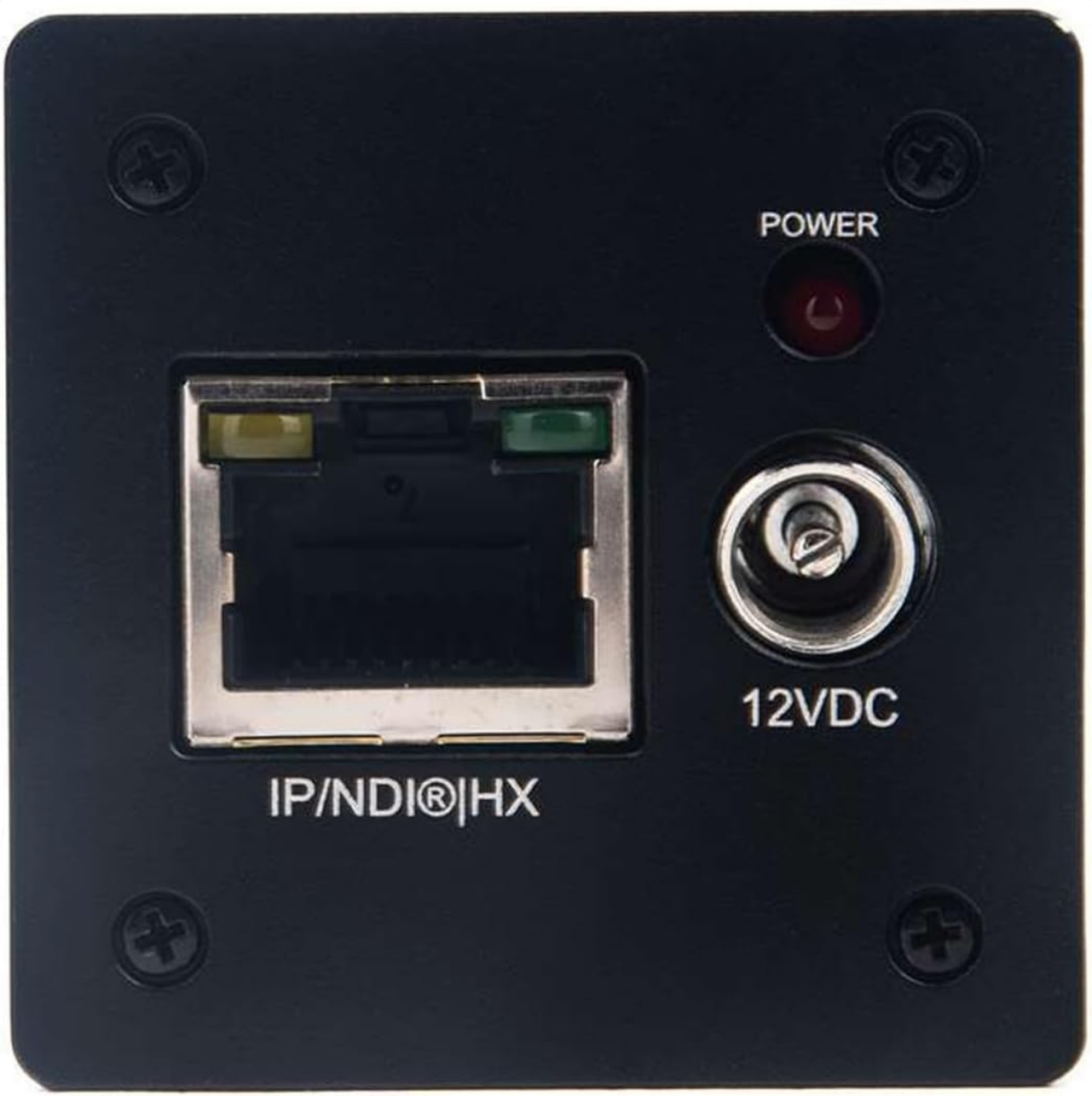
Figure 2: Rear panel of the AIDA HD-NDI-Cube, showing the IP/NDI|HX Ethernet port and 12VDC power input.
