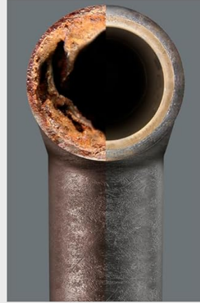
Pipe Corrosion and Buildup
