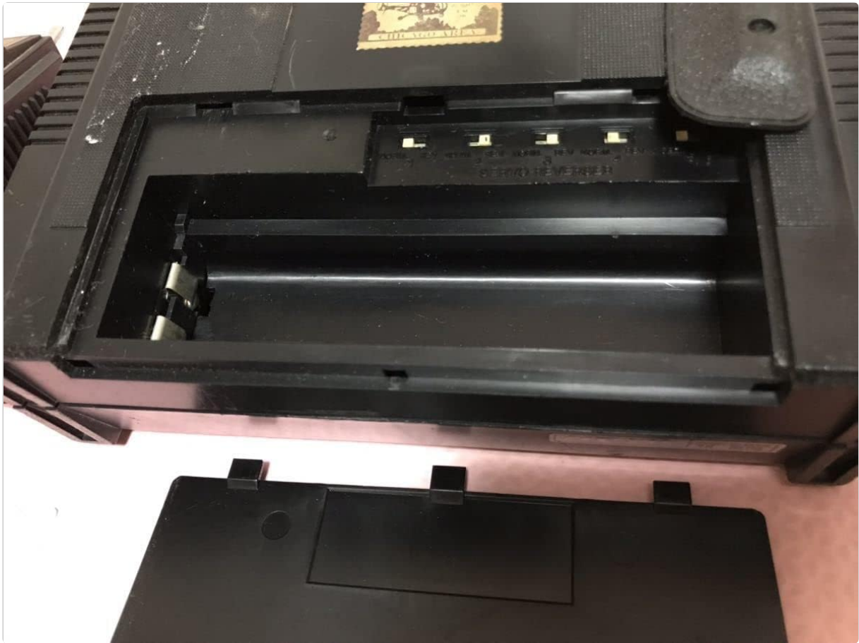
Figure 3: Another view of the open battery compartment of a FUTABA Challenger RC controller. This angle provides a clearer view of the "SERVO REVERSER" switches located above the battery slots, indicating channels for servo reversal settings.
