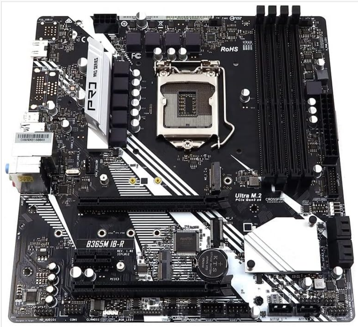
Figure 2: Top-down view of the B365M IB-R Motherboard. This perspective clearly shows the Intel B365 chipset heatsink, SATA
