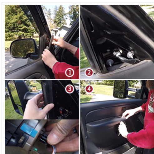
Figure 5.3: Visual guide to the installation process, from removing the old mirror to connecting the new one.
