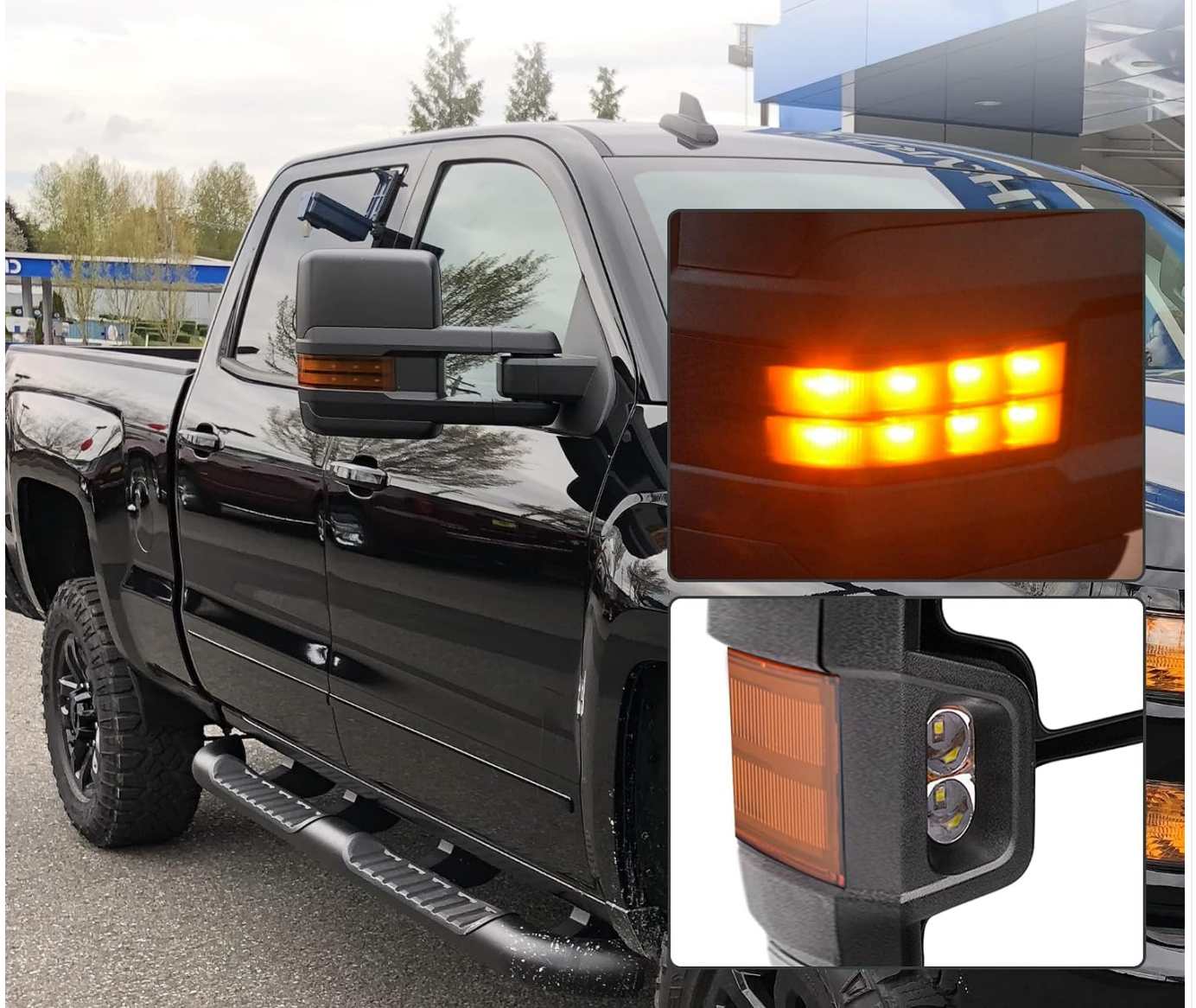
Figure 2.3: Bright LED light source for turn signals, enhancing visibility to other road users.
