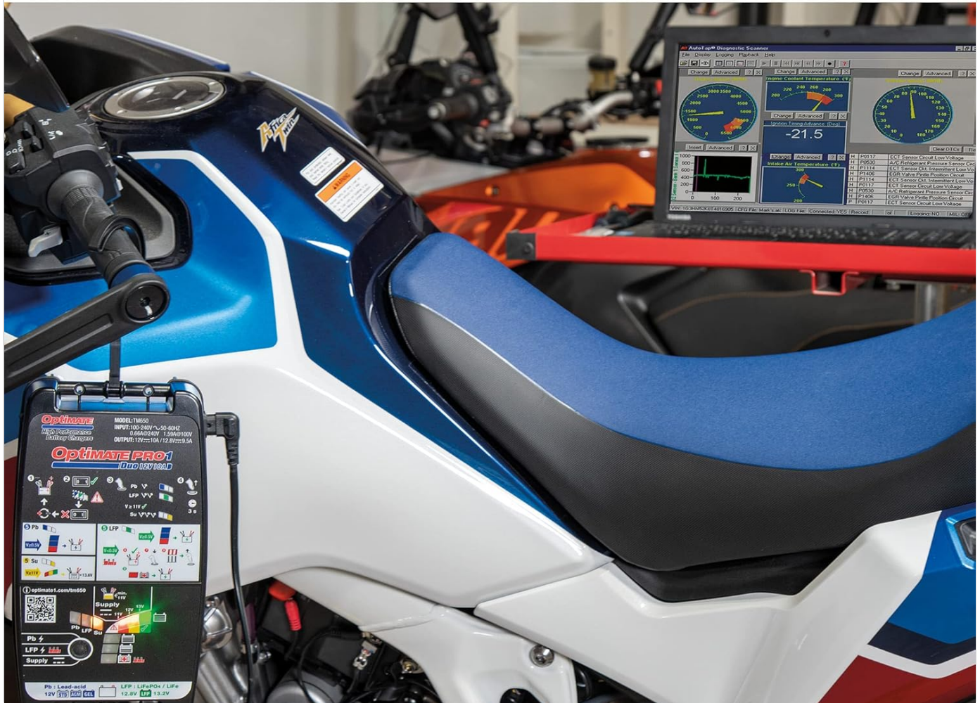
Figure 5: The PowerSupply mode maintains stable voltage for vehicle electronics during adjustments or software updates.
