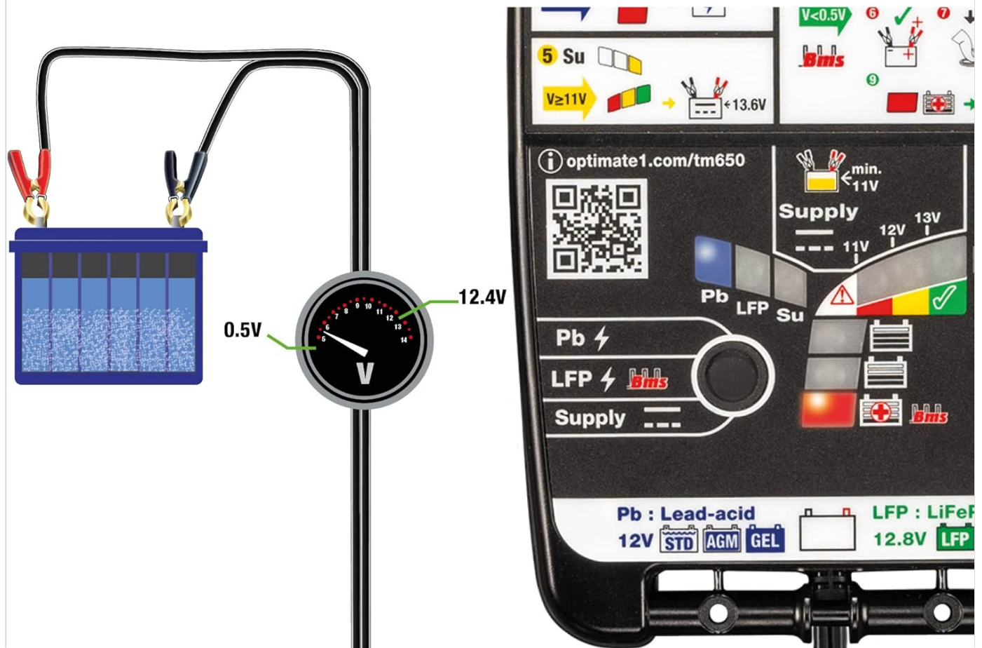
Figure 6: Illustration of the smart recovery process for deeply discharged batteries, showing voltage measurement.
