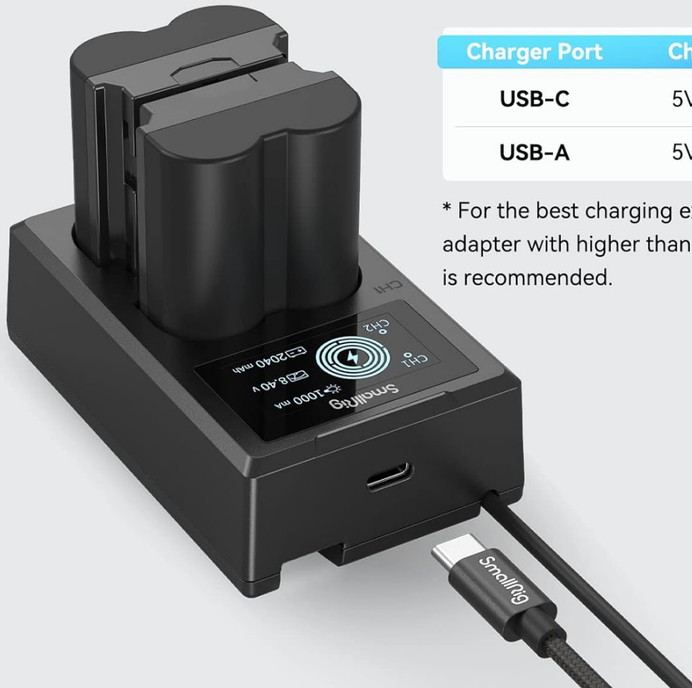
Figure 3.2: The charger's input specifications for USB-C and USB-A are both 5V/2.1A (minimum). For optimal charging, a power adapter with higher than 5V/2.1A output is recommended.
