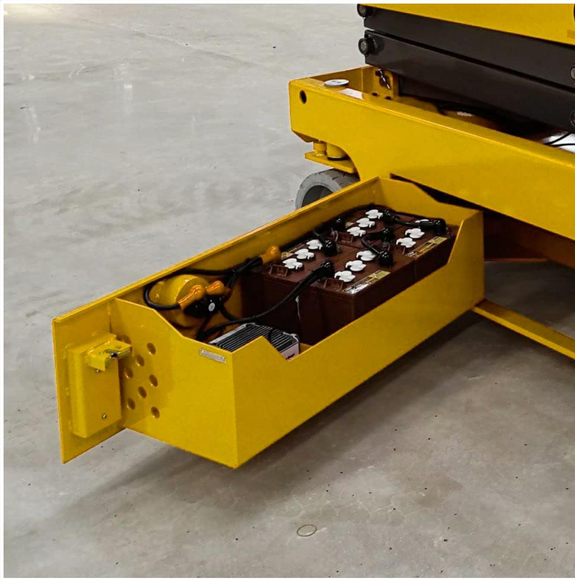
Image 4: The battery charger shown installed within the battery compartment of a yellow scissor lift, demonstrating a typical installation scenario.
