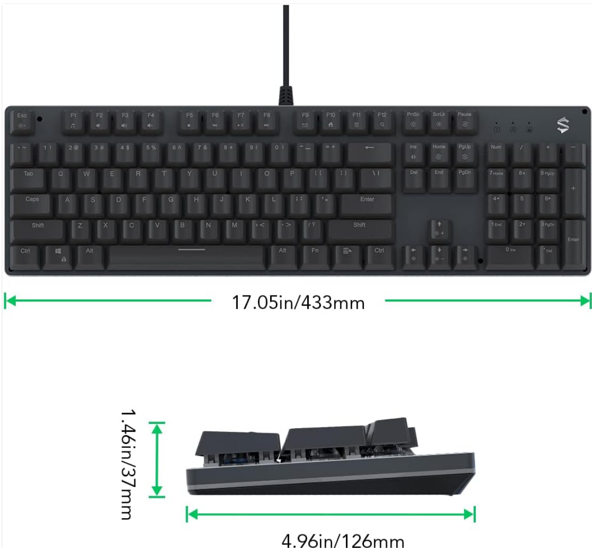
Image: Technical drawing showing the dimensions of the Black Shark Sixgill K2 keyboard.
