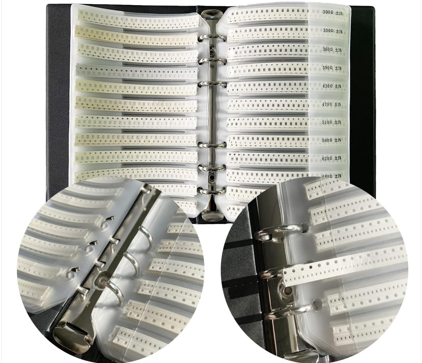
Figure 3: Detail of the ring binder and resistor strip organization.
