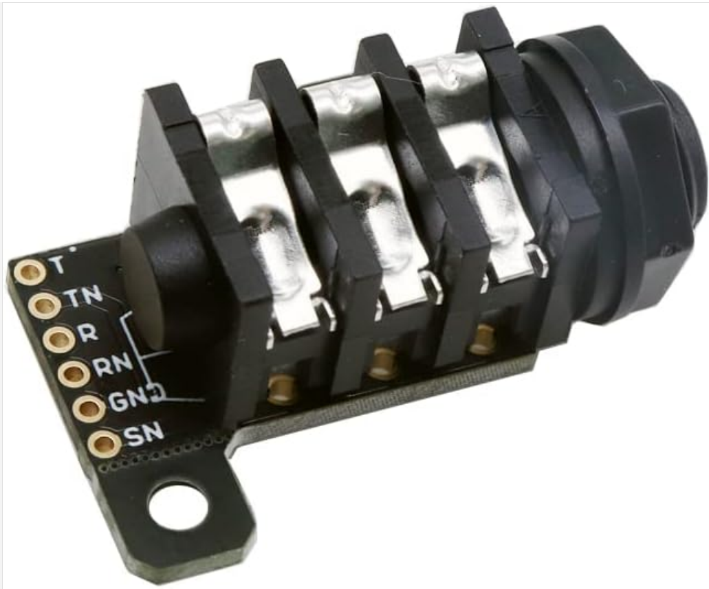
Image: A close-up view of the Treedix TRS Jack Breakout Board, showing the 1/4" female socket and the labeled breakout pins (T, TN, R, RN, GND, S, SN) on the PCB.
