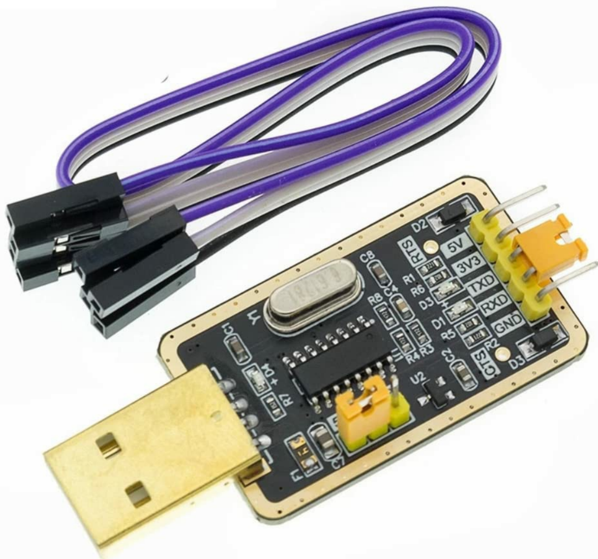
Figure 1: Overall view of the Fasizi USB to TTL converter module. This image shows the compact design, including the USB-A connector on one end and the pin headers for serial communication on the other. The main CH340G chip is visible in the center.
