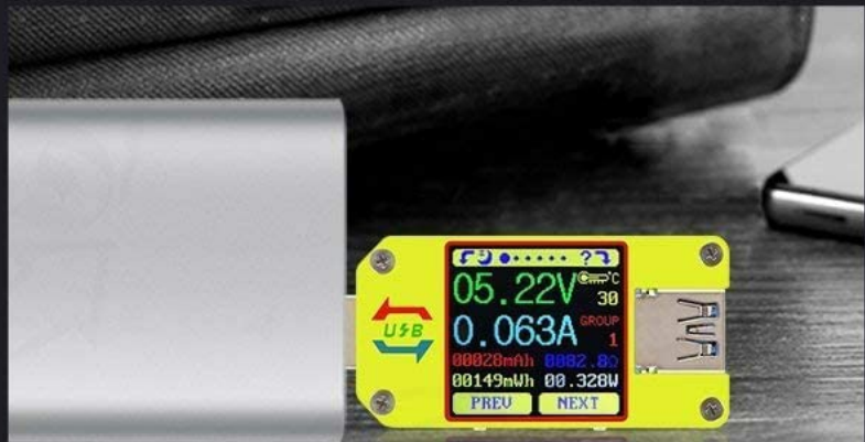
Figure 6: The UM34C screen showing quick charge recognition and various detection modes for comprehensive analysis.
