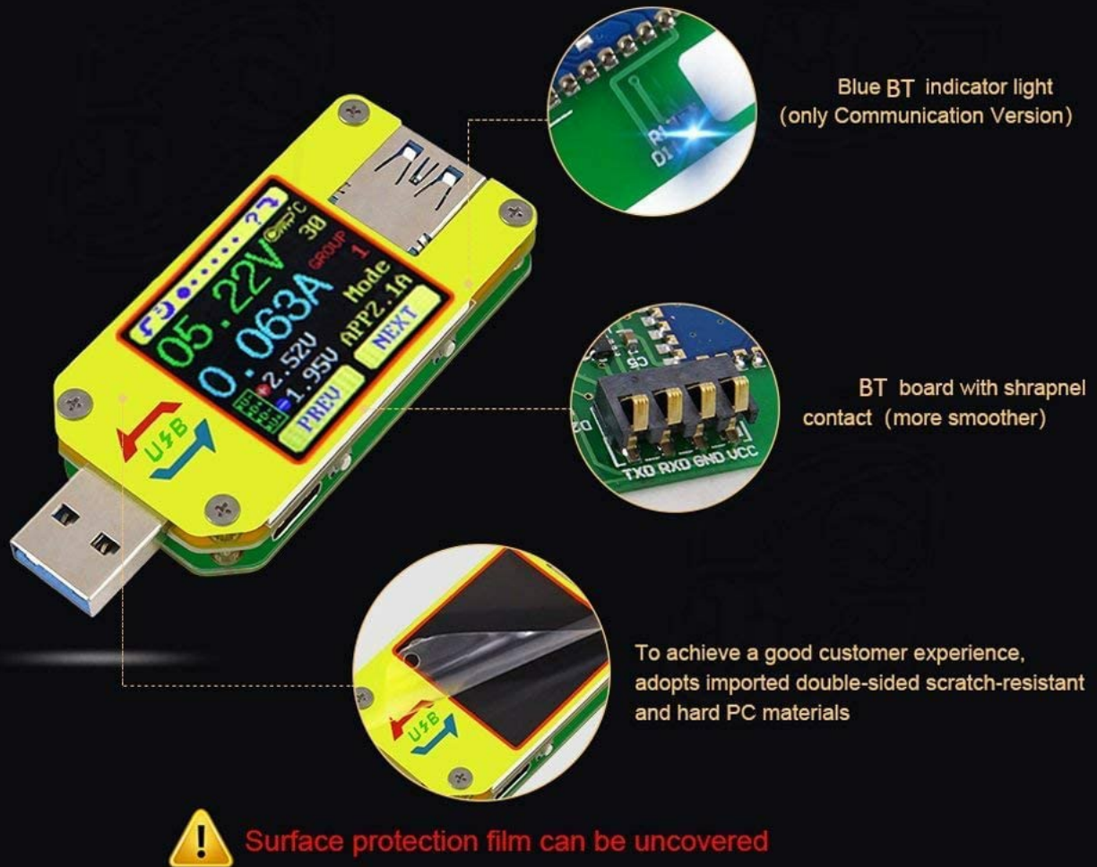
Figure 7: An illustration of the UM34C's internal components and design features, including the Bluetooth indicator light and durable PC materials.
