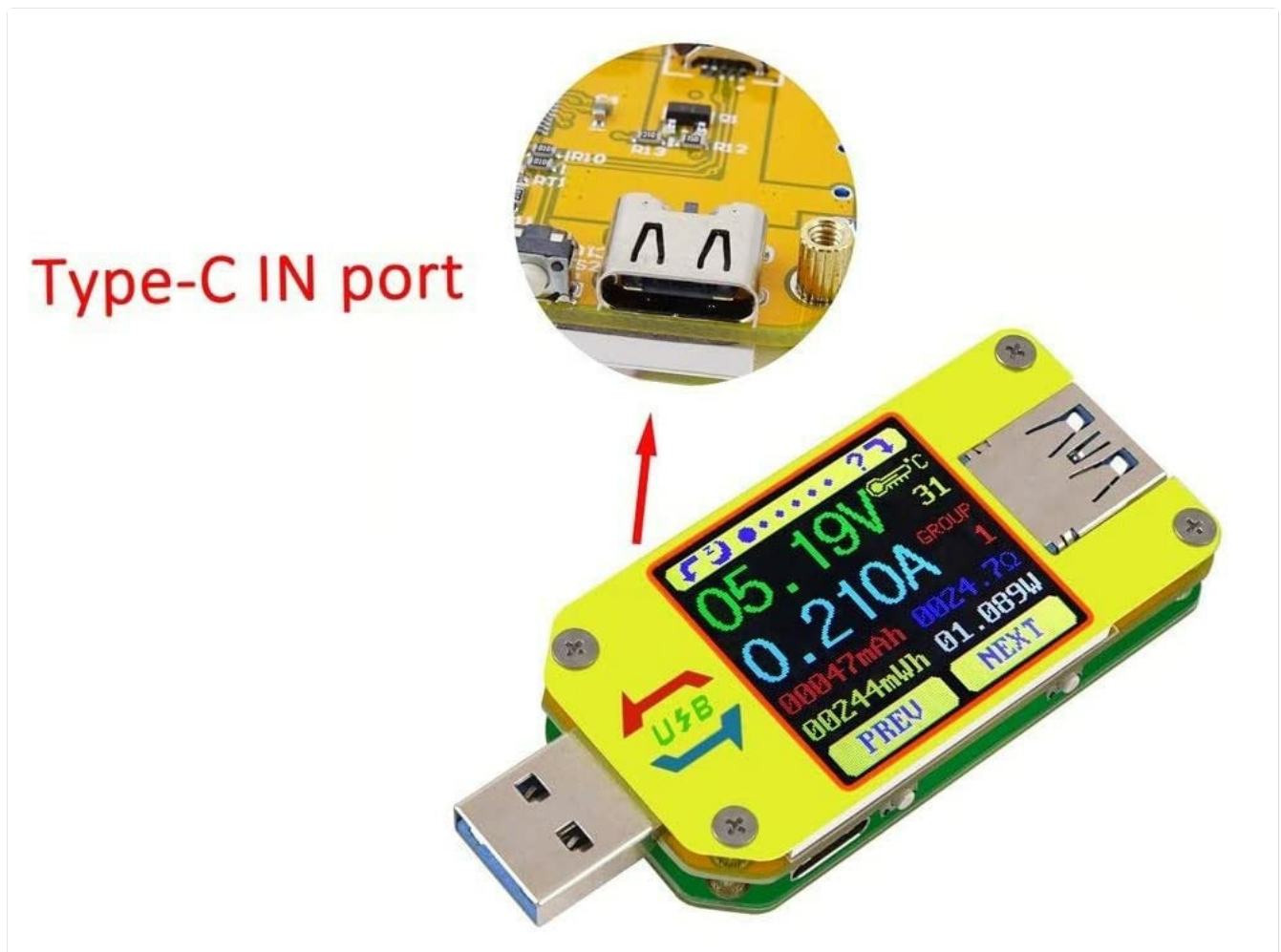
Figure 2: Detail of the Type-C IN port, allowing connection of Type-C devices for testing.
