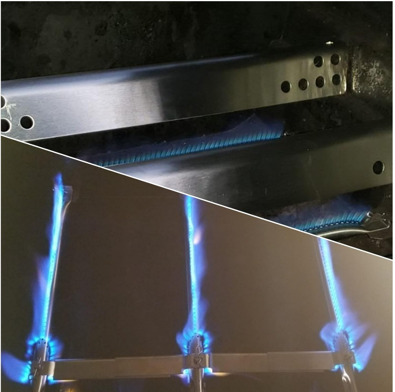
Image: Visual representation of proper flame distribution and heat plate function after installation.
