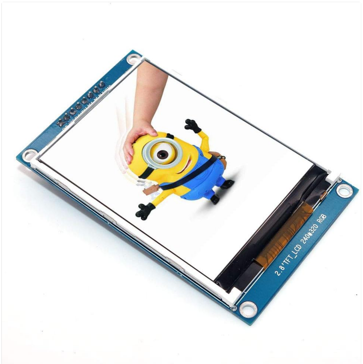
Figure 4.1: The Fasizi 2.8-inch TFT LCD SPI Module displaying an example image, demonstrating its color capabilities.
