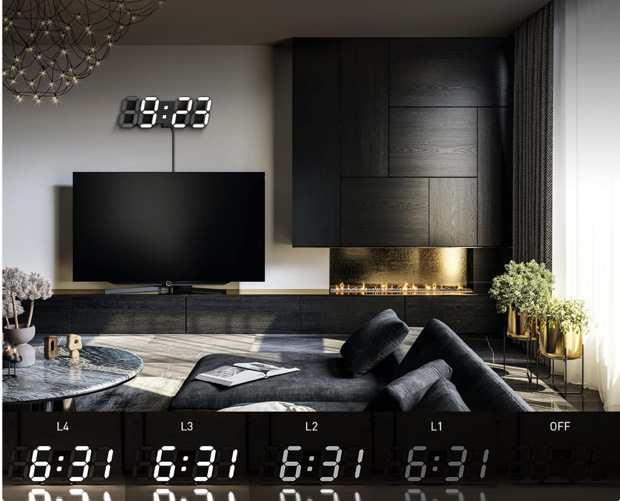
Image 4.1: Illustration of the clock's four brightness levels (L4, L3, L2, L1) and the OFF state, demonstrating how the display intensity changes.
