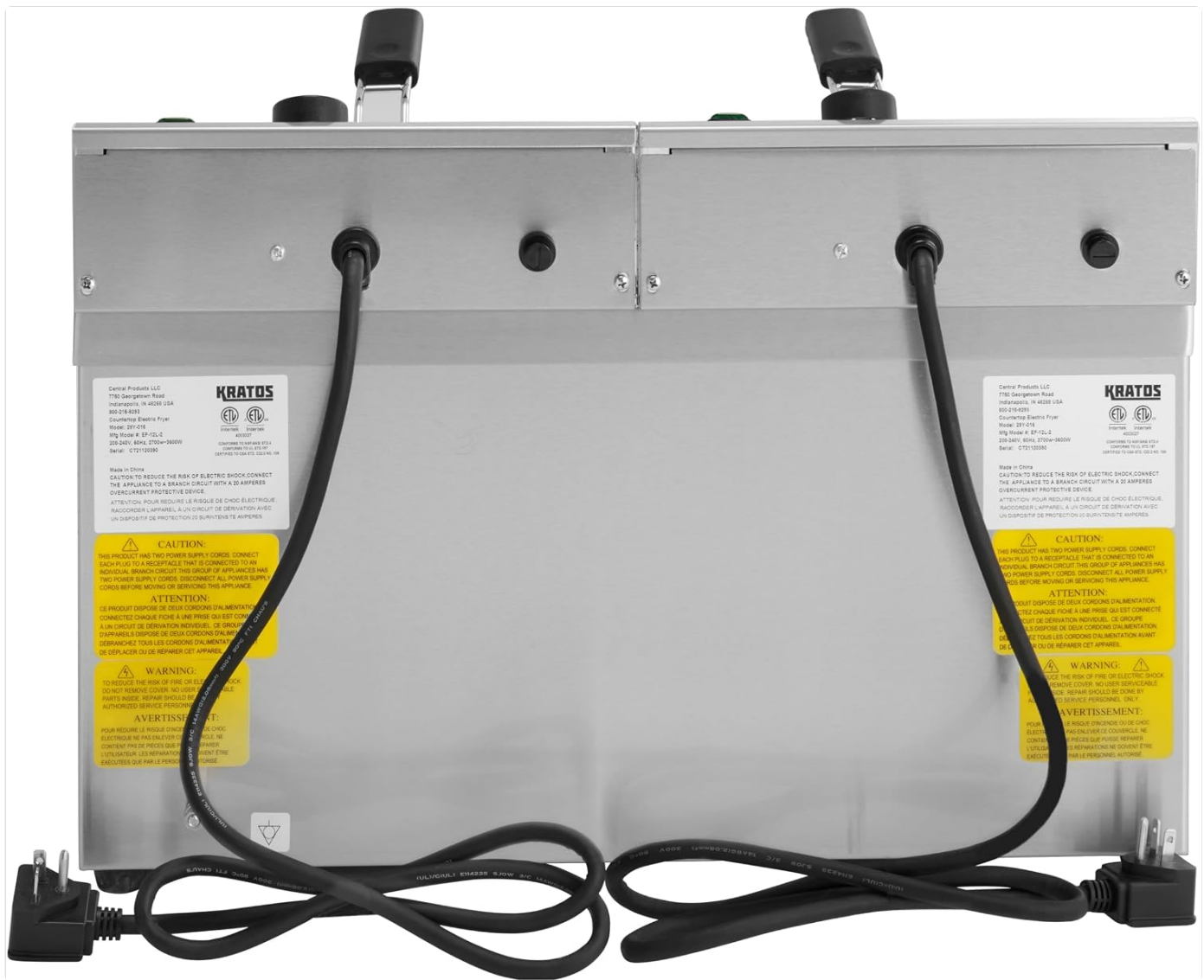
Figure 2: Rear Electrical Connections. This image shows the back of the fryer with its two power cords, each terminating in a NEMA 6-20P plug, indicating the dual electrical requirements for independent tank operation.
