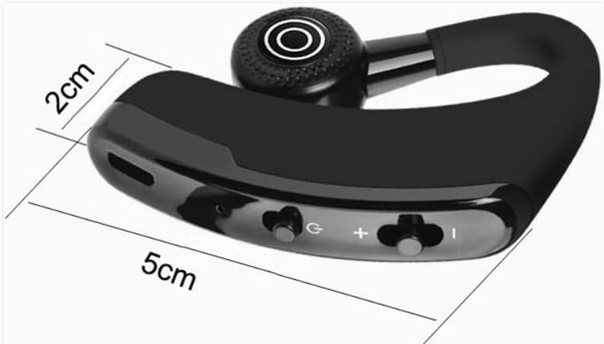
Image 3.1: Headset diagram showing approximate dimensions (5cm length, 2cm width) and control button locations (Power, Volume Up, Volume Down).
