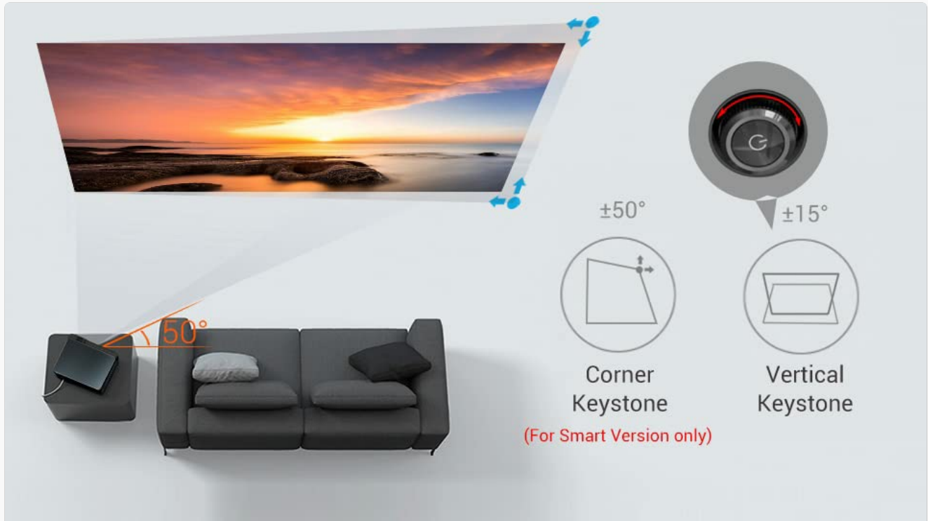
Image 2.3: Diagram illustrating vertical and corner keystone correction capabilities.
