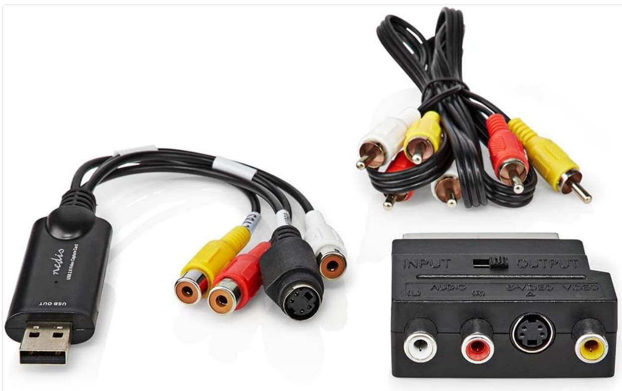
Image 1.1: The Nedis VGRRU101BK USB 2.0 Video Grabber, showing its USB connector, RCA (yellow, white, red) and S-Video input ports, and an included SCART adapter. This device facilitates the conversion of analog video signals to digital format for computer storage.
