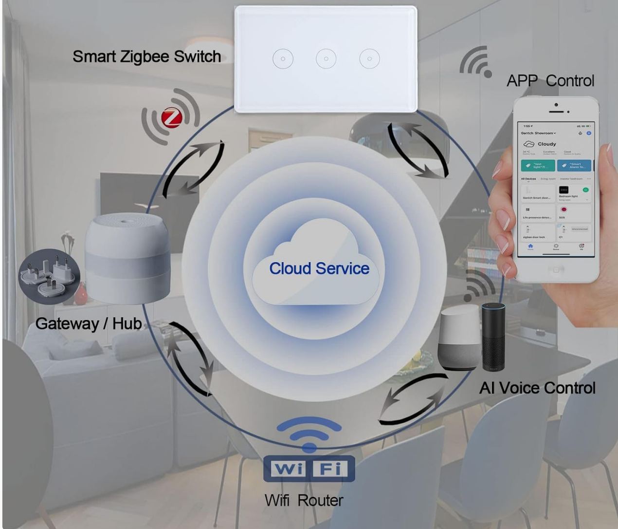
Image: Diagram illustrating how the Smart Zigbee Switch connects to a Gateway/Hub, which then connects to a WiFi Router and Cloud Service. This enables App Control and AI Voice Control (e.g., Alexa, Google Home).
