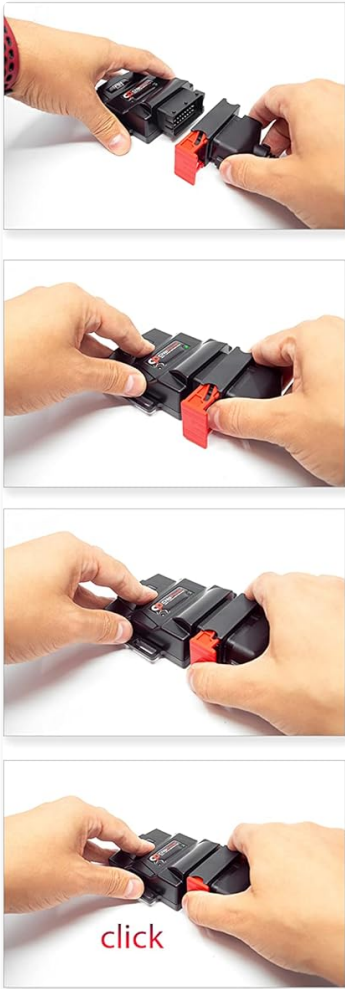
Image: Visual guide demonstrating the connection process of the module's cable to the vehicle's wiring harness, ensuring a 'click' for a secure fit.
